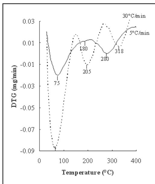
**Fig. 3** TPD profiles of phenol on MgO (calcined from Mg(OH)<sub>2</sub> at 600°C) by the TG method with a ramp rate of 5°C/min and 30°C/min.
