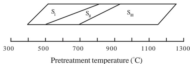
**Fig. 7** Three types of sites on MgO with increasing pretreatment temperature (26).
