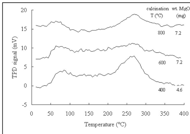
**Fig. 2** TPD profiles of phenol on MgO samples using TCD detector.
