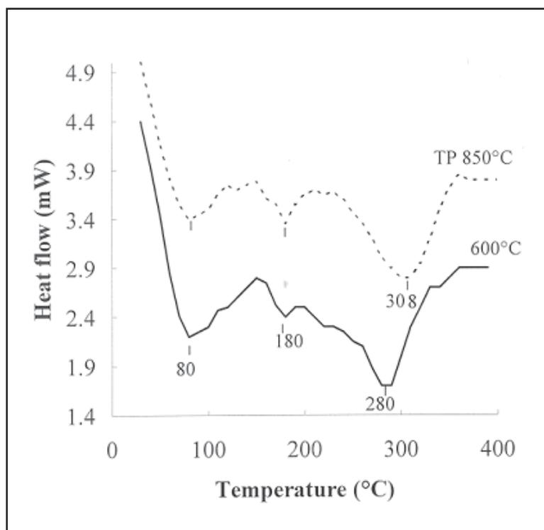
**Fig. 4** TPD profiles of phenol desorbed from MgO calcined at 600 and 850°C.
