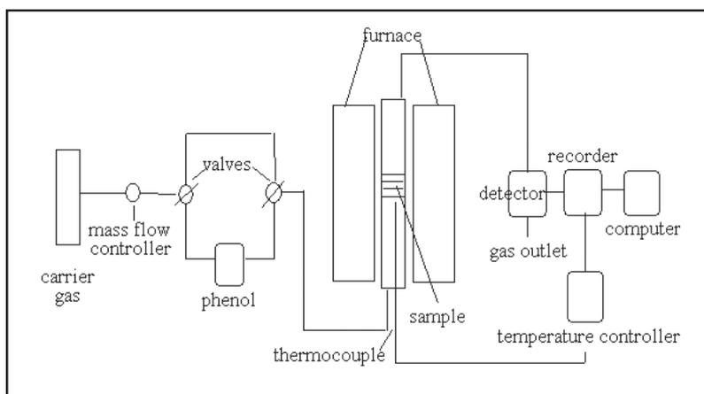
**Fig. 1** TPD apparatus with thermal conductivity detector(TCD).
