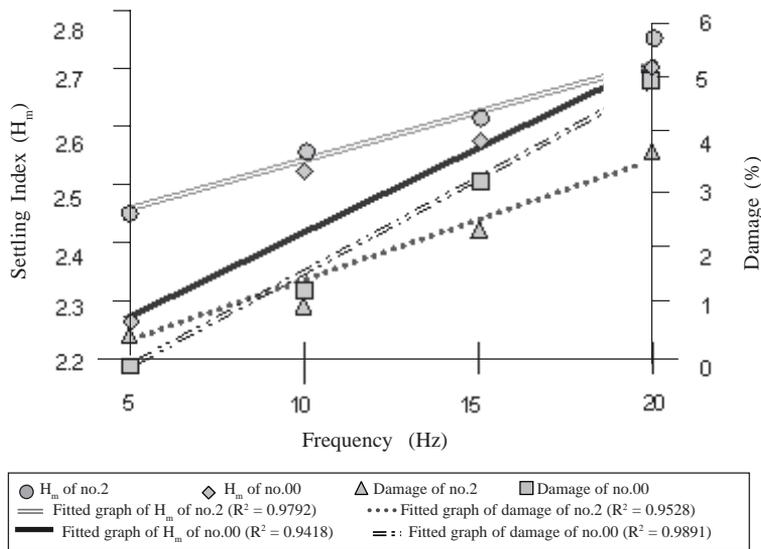
**Fig. 3** Graphs fitted by linear regression between  $H_m$  and damage vs. frequency.
