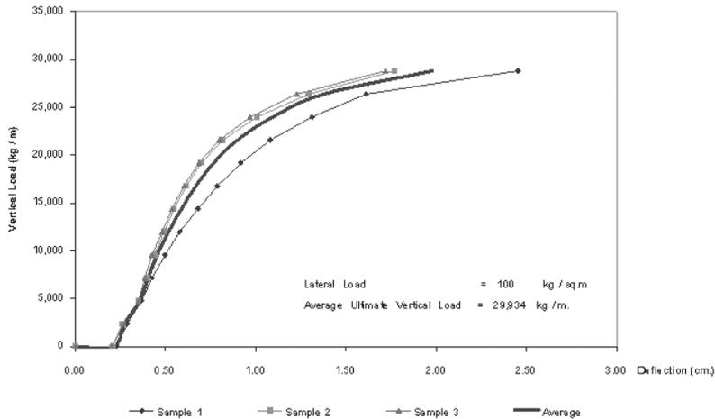
**Fig. 3** The correlation between ultimate vertical load (kg/m) and deflection (cm) of SIP specimens.
