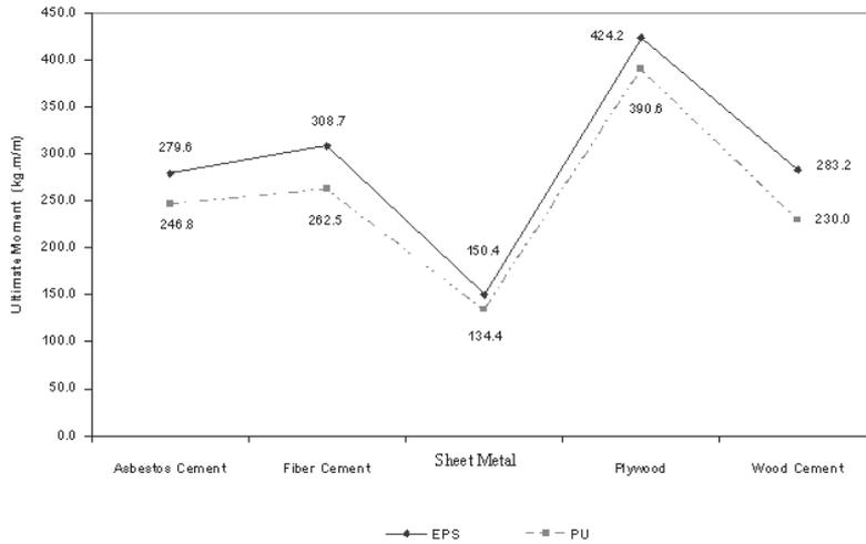
**Fig. 2** Average ultimate bending moment (kg-m/m) of SIP specimens using different composite materials.<sup>5</sup>
