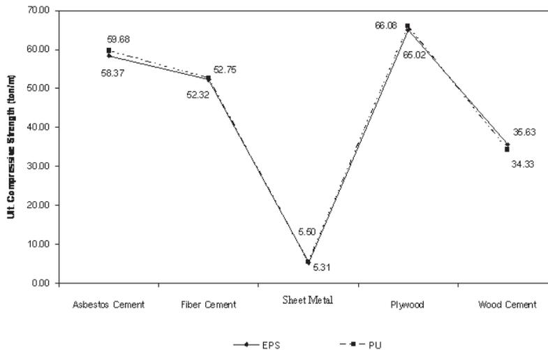
**Fig. 1** Average ultimate compressive strength (ton/m) of SIP specimens using different composite materials.<sup>4</sup>
